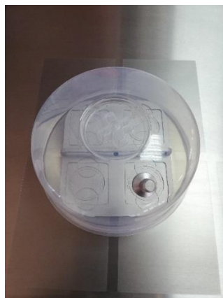
Figure 11.8 Gas hood placed over the gas nozzle
