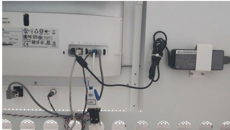
Figure 34.7 Cable connection in the back of the Multi-zone ART Workstation
